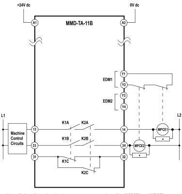
\* Installation of transient (arc) suppressors across the coils of MPCE1 and MPCE2 is recommended (see Warning)
