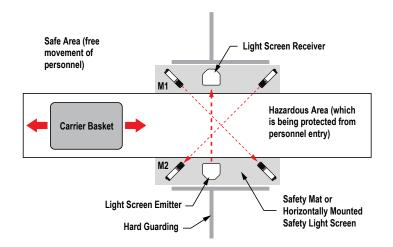
Figure 36. X-Pattern Entry/Exit system using two pairs of opposed-mode photoelectric muting devices
