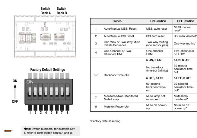
Figure 4. Muting Module manual configuration parameters
