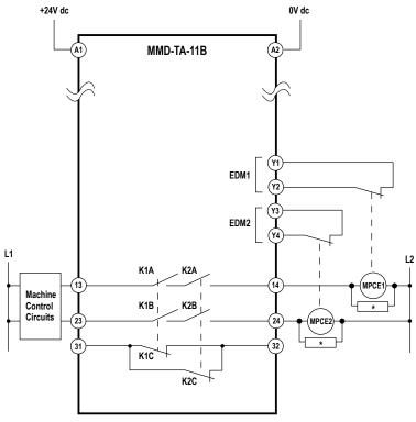
\* Installation of transient (arc) suppressors across the coils of MPCE1 and MPCE2 is recommended (see Warning)
