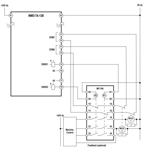
\* Installation of transient (arc) suppressors across the coils of MPCE1 and MPCE2 is recommended (see Warning) Figure 31. Generic machine interface wiring, model MMD-TA-12B: interface module with two-channel EDM
