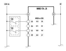
Figure 18. MSSI and SSI Category 3 interfacing: two positive-opening switches per single guard
