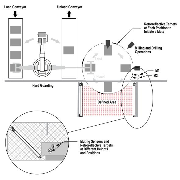
Figure 43. A typical application for turret table inspection or operation station muting, using retroreflective photoelectric sensors as muting devices
