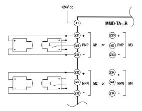
Figure 10. Relay (hard contact) output sensors
