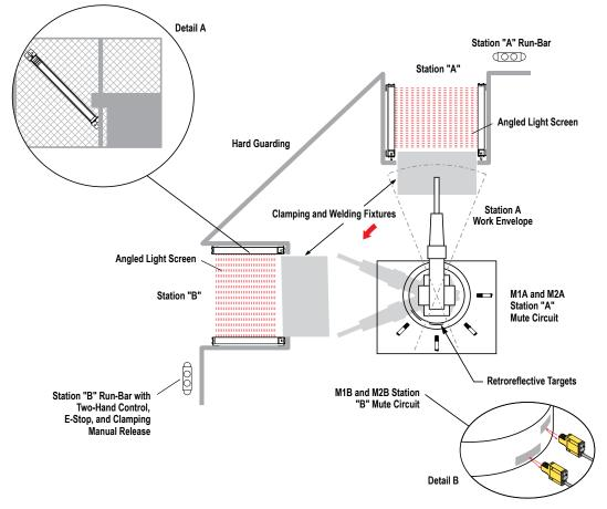
Figure 42. A robot load/unload application with two-station home-position muting, using polarized retroreflective photoelectrics as muting devices
