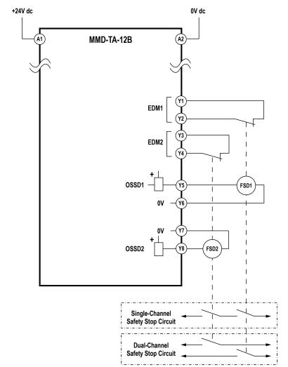
Figure 30. Generic machine interface wiring: module model MMD-TA-12B, FSD with Two-Channel EDM
