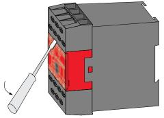
Figure 7. Removal of Terminal Blocks
