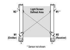
Figure 38. Photoelectric muting devices placed diagonally
