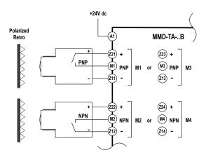
Figure 11. Two (or four) sensors using semiconductor outputs
