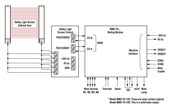
Figure 1. Block diagram of a safeguarding system employing the Muting Module and a safety light screen (user-supplied) as a primary safety device
