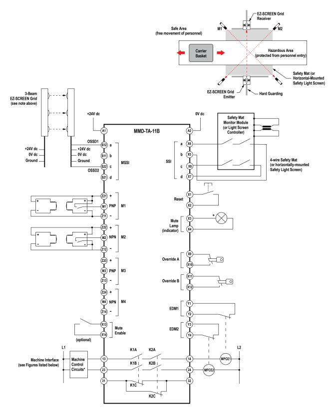
Machine interface - see *Figure 27* (p. 35), *Figure 28* (p. 36), *Figure 30* (p. 41), and *Figure 35* (p. 45). *Figure 29. Interfacing supplemental safeguarding to prevent personnel from entering the hazardous area during the mute*
