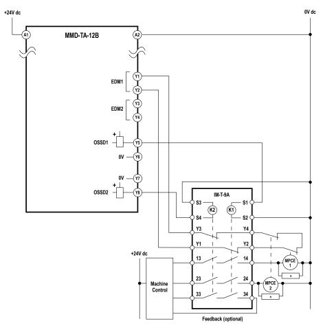
\* Installation of transient (arc) suppressors across the coils of MPCE1 and MPCE2 is recommended (see Warning) Figure 32. Generic machine interface wiring, model MMD-TA-12B: interface module with one-channel EDM
