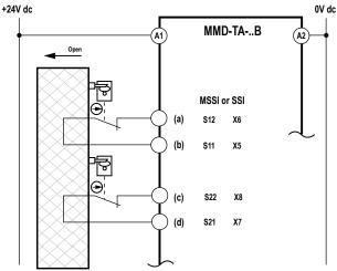
Figure 28. SSI Category 4 interfacing: positive-opening interlocking switch(es)
