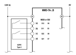
Figure 22. MSSI and SSI Category 4 interfacing: category 4 safeguarding device with relay outputs (for example, MINI-SCREEN or AOPD Type 4 per IEC 61496-1/-2)
