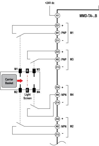
Figure 9. Four Limit Switches as M1, M2, M3, and M4
