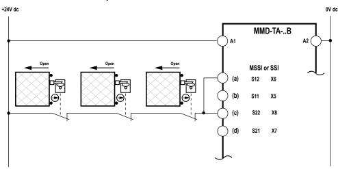
Figure 26. MSSI or SSI Category 2 interfacing: positive opening
