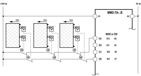
Figure 27. MSSI or SSI Category 3 interfacing: Positive-opening Interlocking switch(es)
