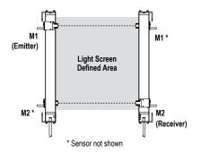
Figure 37. Horizontal photoelectric muting devices placed at different heights
